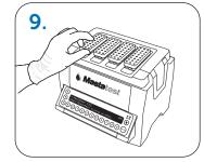
Insert cartridge into Lapbox with the arrows facing to the back, and replace the lid
